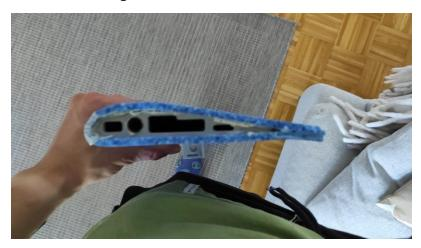
I followed the same process for the fuselage, printing out parts to fit the carbon tubes and foam.
